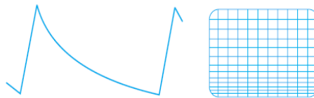
Fig. 19.3 (b). Non-linear sawtooth causing crowding of lines at the bottom of the raster.
