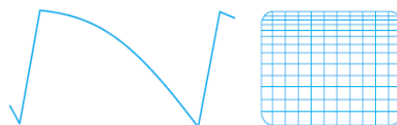
Fig. 19.3 (c). Non-linear sawtooth causing crowding of lines at the top of the raster.
